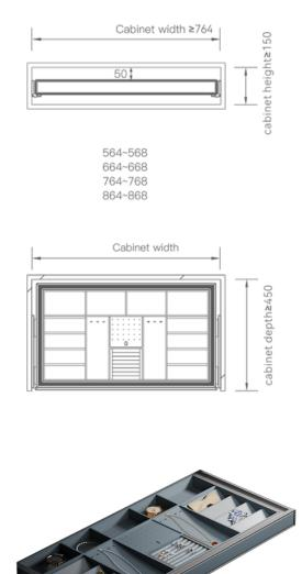
Aluminum frame; front side is of seamless connection.
